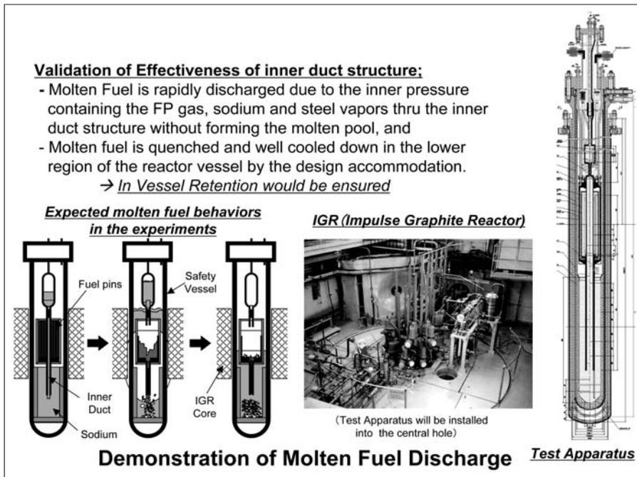
Fig. 8. Aim; Demonstration of the re-criticality free mechanism due to early molten fuel discharge to the outer region.
